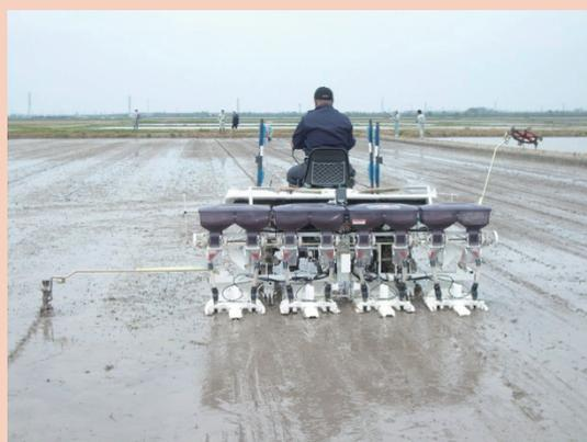
Direct sowing cultivation (A multipurpose rice transplanter equipped with a sowing machine)
