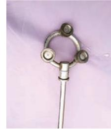
Nozzles commonly used in insecticide spraying
